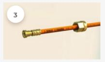
When pushing the ferrule over the hose end, ensure its correct positioning, in line with the hose end. Push the insert into the hose end you want to assemble.
