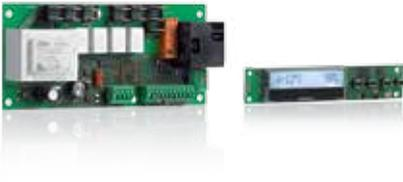
**Custom solution in split version, with LCD display and mechanical keys**
