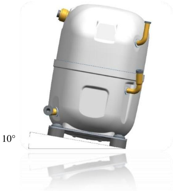
Before soldering the oil equalization tube for AJP compressors, tilt the compressor by at least 10° as shown.
